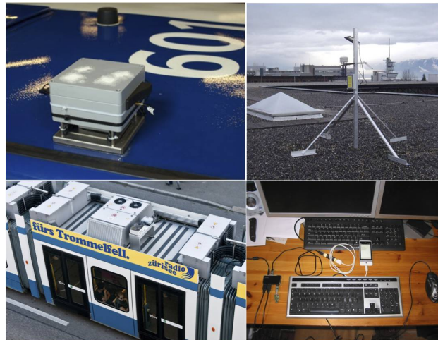
Fig. 1. OpenSense air pollution sensors that could be used in community sensing. Top left: on top of a bus; bottom left: on top of a tram; top right: attached to a solar-powered weather station on a building; and bottom right: attached to a smartphone.
